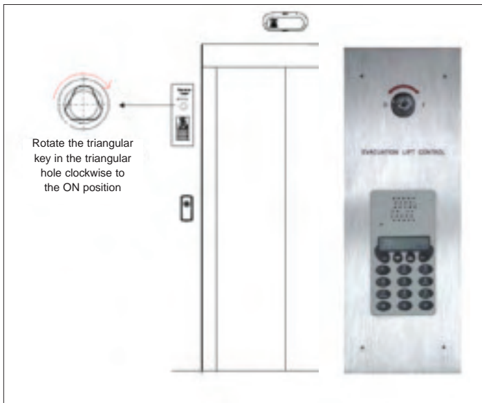
Figure 4: Elevator evacuation control switch at the main exit floor (along with master station of elevator evacuation communication system) (Courtesy: Drucegrove, the U.K.)
